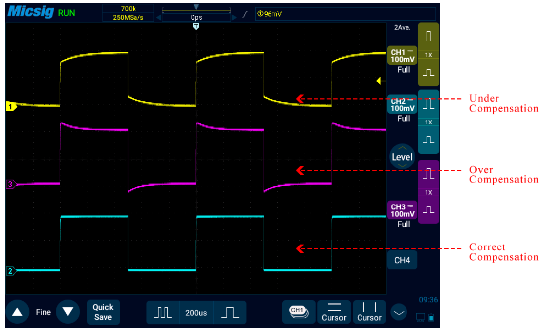
Figure 2-14 Probe Compensation
