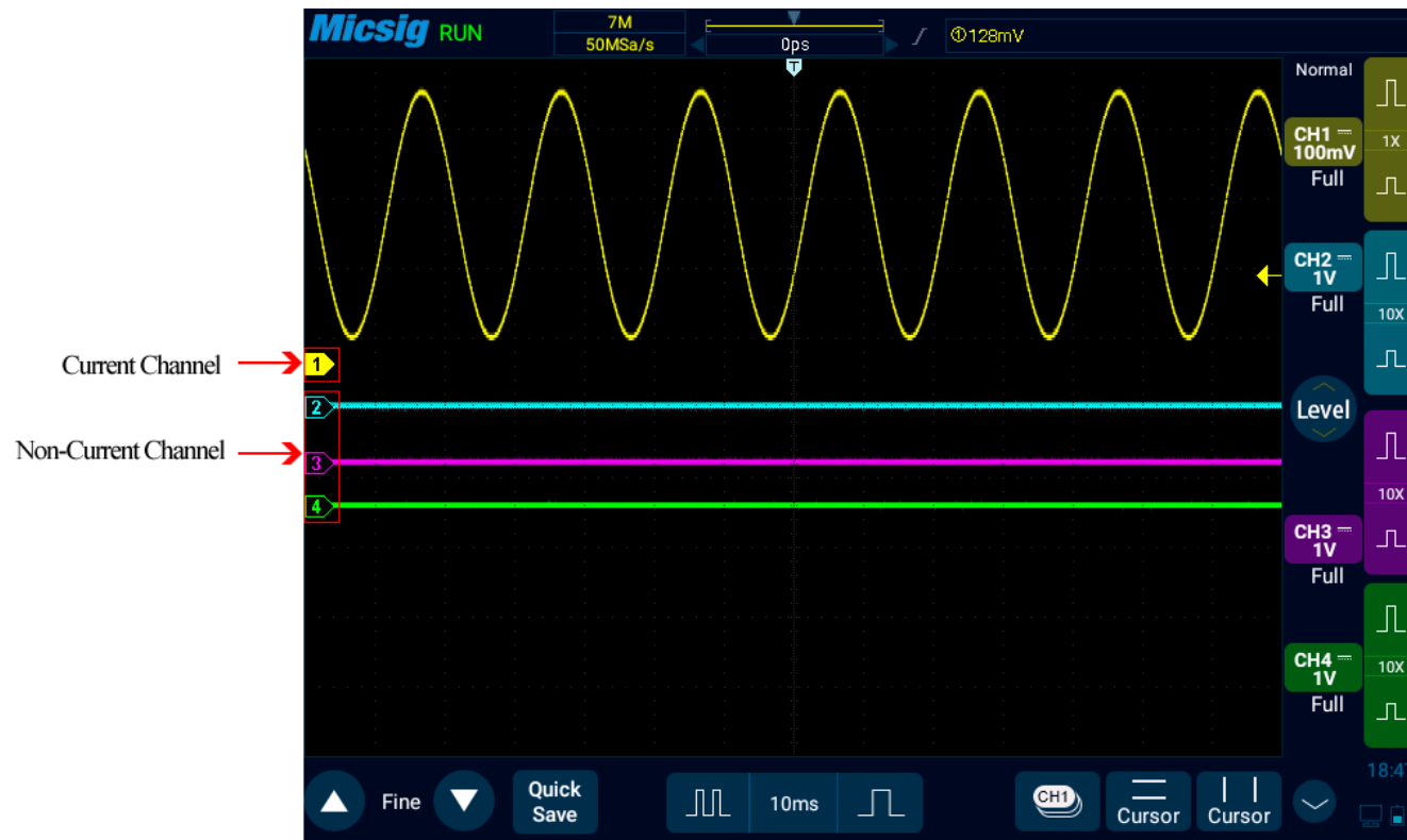
Figure 5-2 Current Channel and Non-Current Channel
