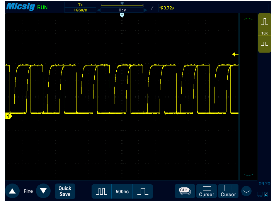
Figure 6-2 Non-Stably Displayed Periodic Signal
